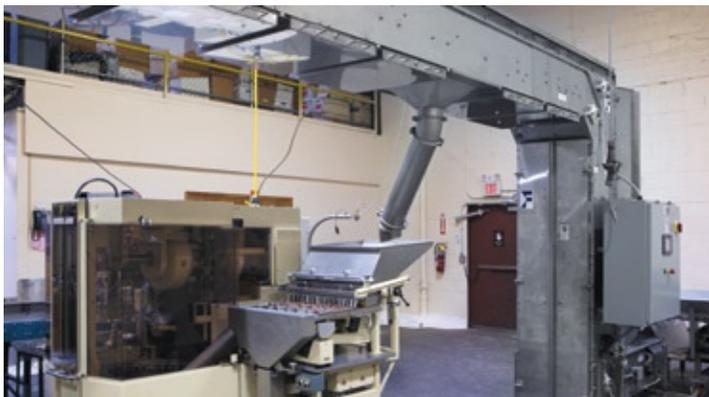
The sorter receives product from the customer’s metal detector on the end of the molding plant line and transfers the product to another Eriez feeder to transfer the product to the elevator/conveyor.
